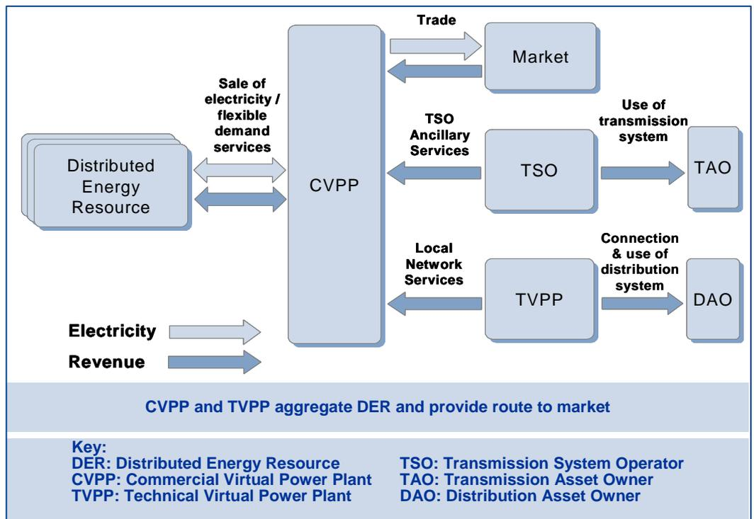
Fig.2 – Contractual structure required
