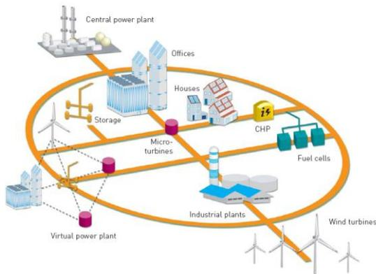
Figure(1) – GD integration to the Smart Grid. [5]
