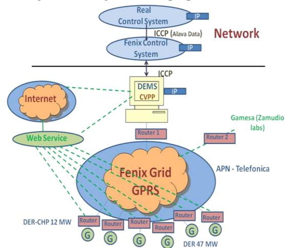
Figure (3)- Demonstration Architecture
