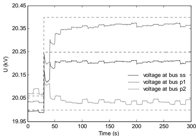
Fig.4. Multi-objective CVC response to multiple set-point step.
